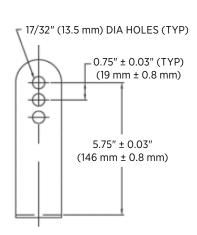
NOTE: MATERIAL SHALL BE 2" (51 mm) WIDE X 1/8" (3 mm) THICK TYPE 304 STAINLESS STEEL
